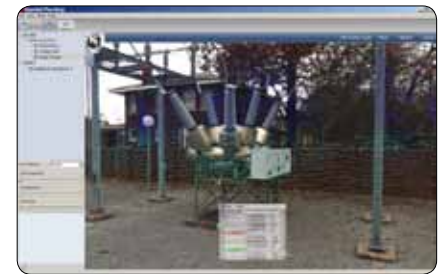
Point Cloud with Image Overlay
