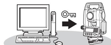
• Turn on the Total Station and press [CHECK] on the user registration screen. The system communicates with the server and the registration is automatically certified.
